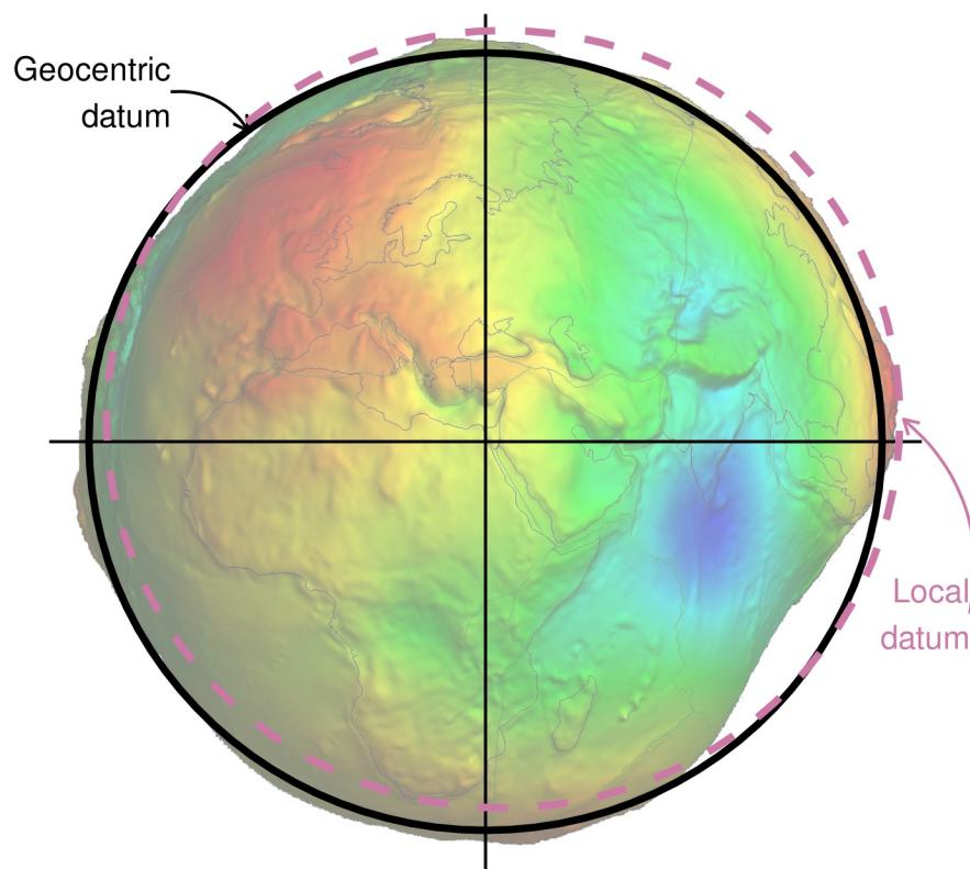
Geocentric and local geodetic datums shown on top of a geoid (in false color and the vertical exaggeration by 10,000 scale factor). Image of the geoid is adapted from the work of Ince et al. (2019).
